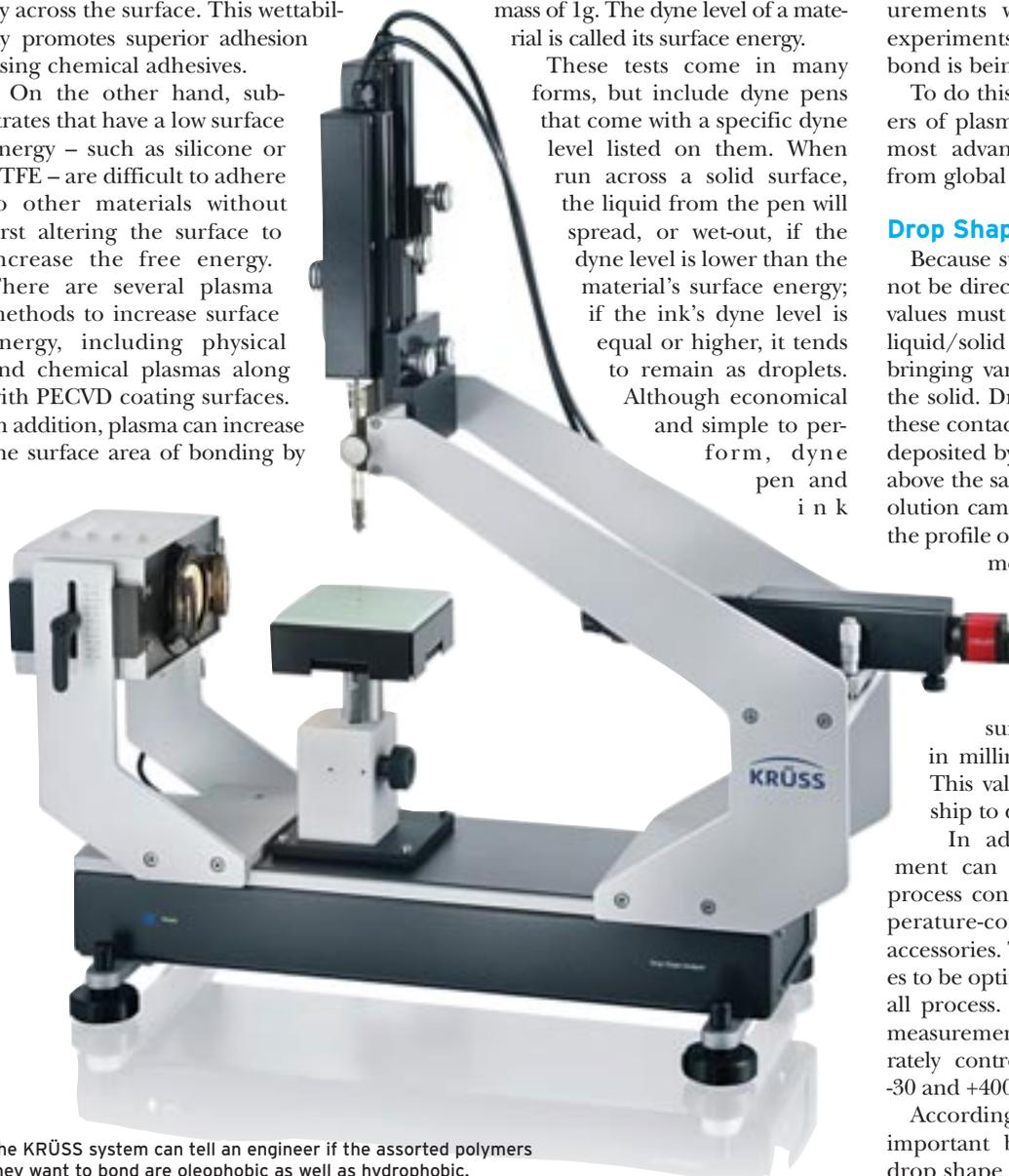
The KRÜSS system can tell an engineer if the assorted polymers they want to bond are oleophobic as well as hydrophobic.
